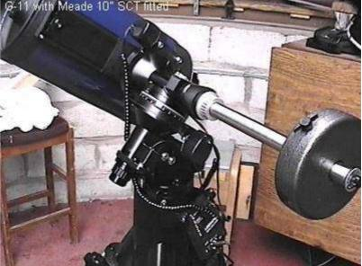
place. The counterweight is a roughly finished cast iron lump, painted in grey hammer finish paint - it doesn't match the rest of the mount.
