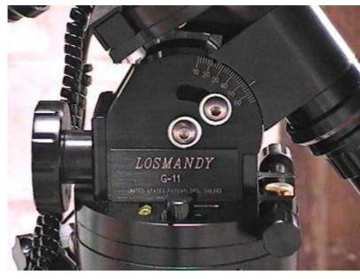
Fitting the SCT onto the mount is straight forward, there are a couple of small hand bolts that stop the dovetail plate sliding off the end. A larger hand wheel bolt secures the SCT's dovetail bar by a vice-like clamp, by slackening this clamp the telescope tube can be slid back and forth to achieve balance on the declination shaft.
