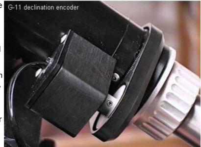
units, geared 2:1, giving 4096 steps per rotation of each axis. There's no mention of how to fit the covers onto the gears. Earlier DSCH units apparently didn't include covers, the fitting sheet hasn't been updated to reflect this.
