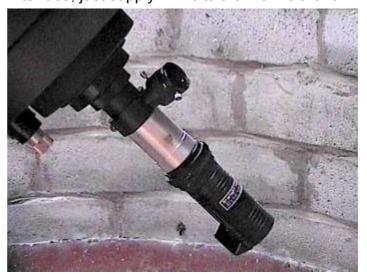
aluminium). The eyepiece projection adapter is fitted with a Canon 'FD' lens series T2 mount, the MX5-C is fitted with a home made Canon FD series camera body plate to M42 thread adapter. This arrangement allows me to swap between a Canon A1 or FTb camera and the MX5-C, it also allows me to use the MX5-C on a variety of Canon lenses. Shown below is the MX5-C alongside a homemade Canon eyepiece adapter.
