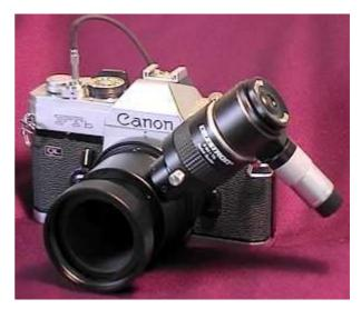
taking a photograph of (this means you can't take a full comet photograph by guiding on the head of the comet), not only that, the adjustment is limited and being off the main optical axis you get anything but sharp points of light from your chosen guide stars!
